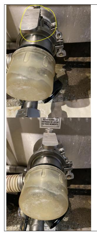
Screw the plastic cap onto the valve assembly as shown. It will screw onto the threads that were revealed when you removed the rubber thread protector in the previous step.
